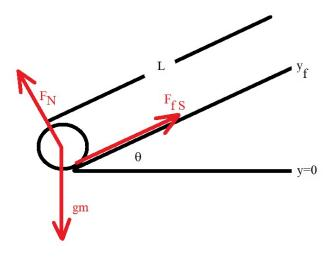
$$0 = \frac{1}{2} m v_f^2 - \frac{1}{2} m v_i^2 + \frac{1}{2} l \omega_f^2 - \frac{1}{2} l \omega_i^2 + g m v_f - g m v_i$$
