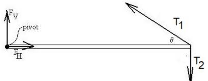
The beam seems to be the central object on which most of the forces of interest act, so to keep track of the forces, draw a free-body diagram.
