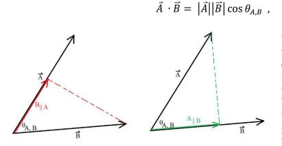
that is, the magnitude of  $\overline{A}$  times the magnitude of  $\overline{B}$  times the cosine of the angle between them if they were placed tail to tail. The dot product is defined to be a scalar. One interpretation of this definition is that we are multiplying the magnitude of  $\overline{A}$ by the component, or *projection*,<sup>8</sup>
