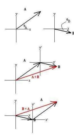
An alternate, but equivalent, method of addition is the parallelogram method. This helps explain the contention of commutativity; the two long sides are
