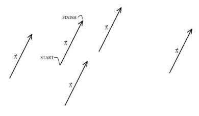
magnetic fields, or nuclear spin. We do need to be careful; once a vector is defined, it has only two properties, magnitude and direction. We can move the vector around as much as we wish so long as those two properties remain constant. For example, in the figure, vector  $\vec{A}$  was constructed to represent the displacement from the START to the FINISH, but all of the other vectors drawn are just as validly vector  $\overline{A}$ .
