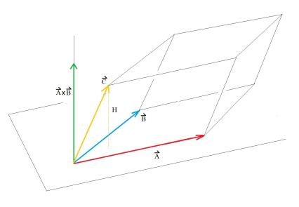
The height H is the projection of  $\vec{C}$  on  $\vec{A} \times \vec{B}$ , so
