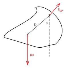
Consider an object of indeterminate shape hanging from an axis, as show. This is known as a *physical pendulum*. D is the distance between the point of suspension and the center of mass. The forces acting on the object comprise a force at the suspension point (the pivot) and the weight, which can be assumed to act at the center of mass. Consider the torques acting on the object when it has been displaced from equilibrium by angle theta:
