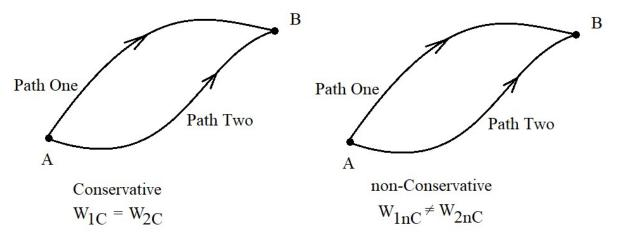
By definition for a conservative force, the work done by the force along any Path One from A to B is the same as along any other Path Two. Since the two paths have only points A and B in common, there must be some numbers associated with the object being at each of these points that
