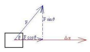
that the components of a vector can replace the original vector. Let's do so for this force. The component parallel to the displacement is F cos  $\theta$  and the component perpendicular is F sin  $\theta$ . The former should contribute to the work, while the latter does not. Sounds like just what we need. Indeed, if the angel were greater than 90°, the cosine would provide the negative sign required when the force and displacement are in generally opposite directions.
