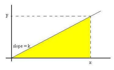
How much work is necessary to stretch (or compress) a spring distance X from its relaxed position? We can use the graphical representation showing  $F_{on spring}$  as a linear function of X with slope k:
