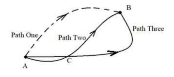
Here we go. Let's start with the work-energy theorem, and divide the works on the left into two categories, depending on whether the associated forces are conservative (C) or non-conservative (NC):
