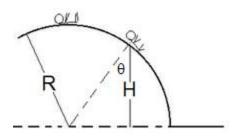
Another classic. Consider a child perched at the top of an igloo, which we will consider to be a hemisphere of radius R covered in slippery snow. He starts with an almost zero speed from the top and travels down the side. At what vertical distance H from the ground will he become airborne?
