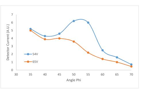
about 50°. For comparison, the 65V curve is also included; the peak is less clear. Accelerating potentials from about 43V to about 66V show some type of peak, however small. By varying the potential and measuring the direction of maximum electron diffraction, we can calculate what wavelength X-rays would have been diffracted in the same direction:
