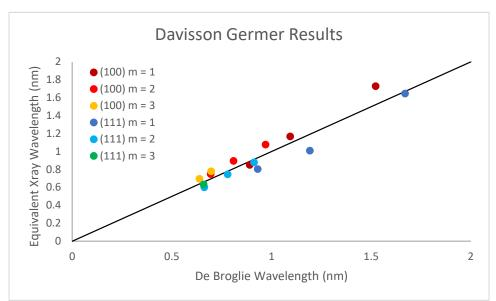
one and shows where the two values would be equal. We can see that the two sets of values are fairly equal to one another, demonstrating that the electrons follow the rule for Bragg diffraction, and therefor behave as waves.
