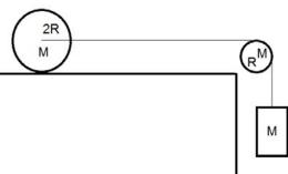
Once released from rest, the cylinder rolls without slipping on the table, and the string does not slip over the disc. What is the linear acceleration of the masses?
