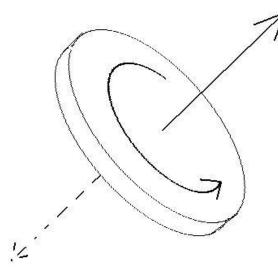
Again, by convention, we'll pick one vector to represent rotation in one direction, and the other to represent the reverse rotation. Use a variation of the *right hand rule* (RHR): curl your fingers in the direction of rotation, and your thumb will point in the direction of the vector  $\Delta \theta$ .
