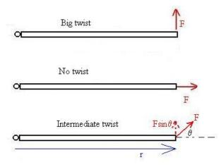
At intermediate angles, it seems clear that we need to take the component of the force which is perpendicular to the r-vector, namely  $Fsin\theta$ , where  $\theta$  is the angle as shown between the force vector and the r vector. So, we might now guess that
