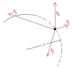
However many forces are applied, they can be added and resolved into components which are either centripetal or tangential, resulting in net force components like this:
